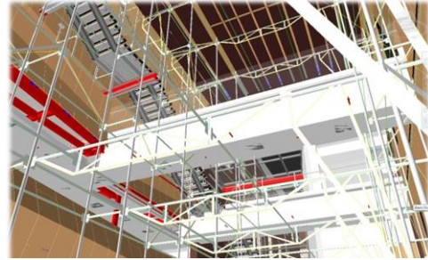
Figure 5 Atrium Scaffolding set-up
