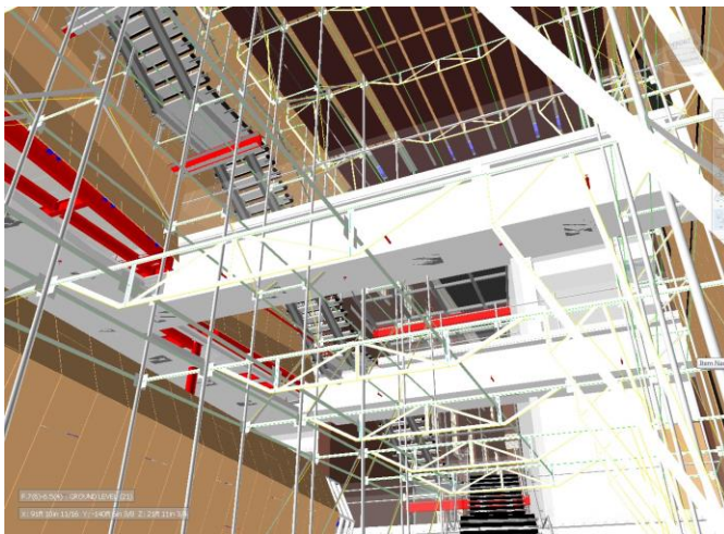
Figure 2 Model depicting the scaffolding set up in atrium2
